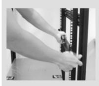
Step 1. Secure the side rails to the rack.
