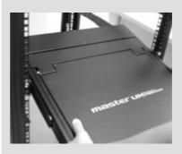
Step 2. Slide the KVM switch onto the rails and secure it to the rack.
