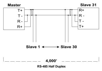
**Note:** When the distance between both ends of the installation is large and/or the transmitted signals aren't stable, insert a 120  $\Omega$  terminal resistor between pins 1 and 2 on the terminal blocks of the two units at each end of the installation.
