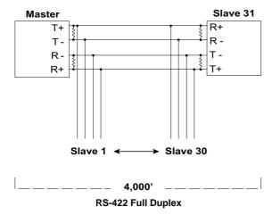
**Note:** When the distance between both ends of the installation is large and/or the transmitted signals are unstable, insert 120  $\Omega$  terminal resistors between pins 1 and 2 and between pins 3 and 4 on the terminal blocks of the two units at each end of the installation.
