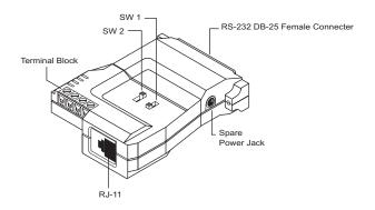
The operating mode, contention control and RS-232C assignments are all configured with two slide switches: SW1 and SW2 (details are given in the *Switch Configuration* section, below).
